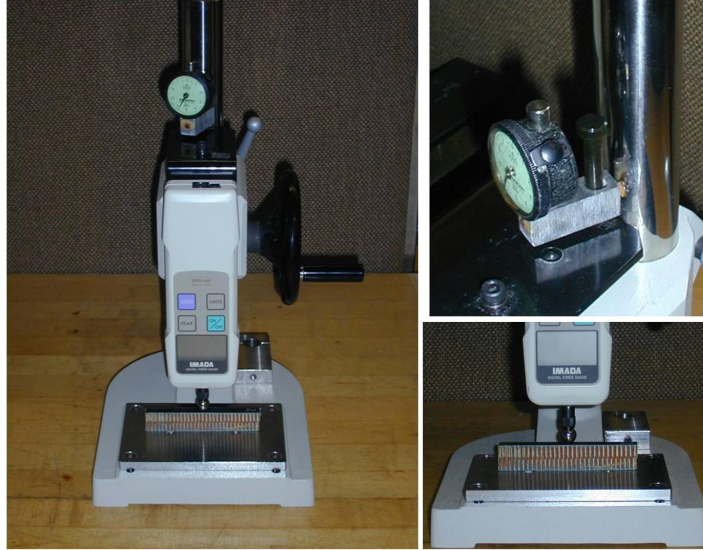
Figure 6.2 Imada loading frame mounted with an Imada force gauge(bottom right) and displacement dial gauge(top right)
