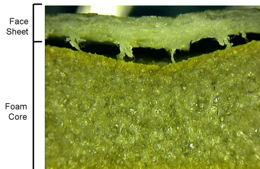
Figure 2.4 Skin-to-core disbond resulting from an impact damage. The structure is composed of a fiberglass face sheet and a Divinycell foam core
